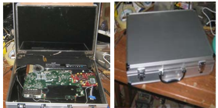
Fig. 6. Assembling of Nomadic Monitoring Unit
